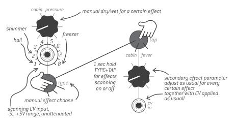
approx. 1.25V per step. If the incoming CV is from -5V to -3.75V, then the first effect type is chosen. If the CV is in the range from -3.75 to -2.5V, then the second effect is chosen and so on, up to the 8<sup>th</sup> effect.
