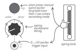
manually by using the TAP button or by applying a trigger into the CABIN FEVER CV input while being in the secondary function. By adjusting the decay to the maximum value, the spring sounds long (up to infinite) with a small self-oscillation. Keep that in mind when you select this effect.
