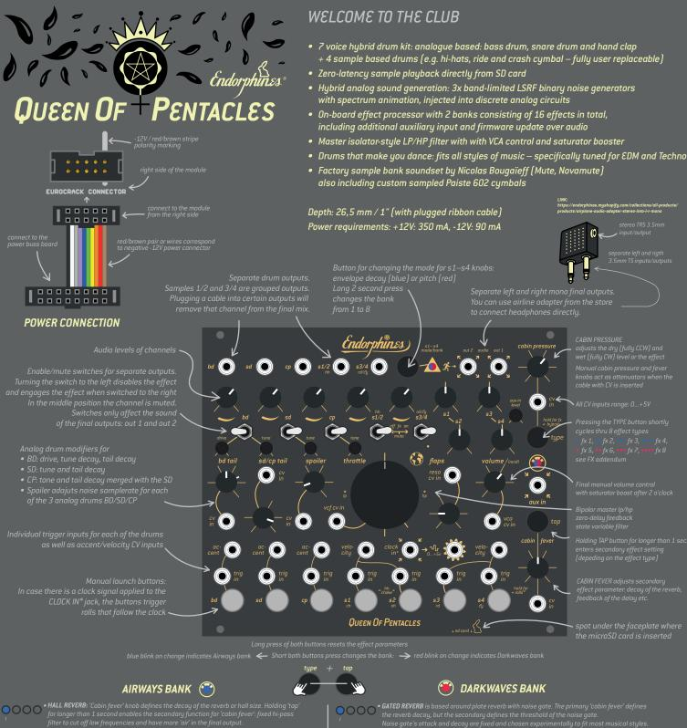
\*SHIMMER REVERB is a variation of the hall reverb with a pitch shifter to create choir-like, huge and unrealistic spaces. The primary 'cabin fever' function defines the decay and the secondary function defines the amount of pitch-shifter mixed into original reverb.
