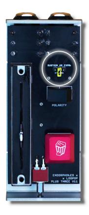
PLUS 3's SUSTAIN side has a hidden feature—a jumper-based selector inside the enclosure (see **SUSTAIN AS EXPR.** yellow jumper on the left photo). By default, PLUS 3's SUSTAIN side is designed to respond to TS-type cables (but also shorting TIP with RING only while using TRS cable). By default the internal jumper isn't connected to anything, it's just "floating" on the middle pin.
