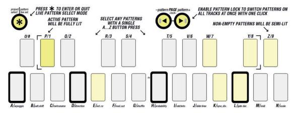
Pressing *LAST STEP* button in live pattern mode will enter the *PROJECT LOAD* menu and you can load any other project with *A...Z* buttons without stopping the sequencer. Loading a new project can be done smoothly on the fly when the current project is still running without losing the sync. Once you press a new project load, after the longest pattern of current project will be finished, all new patters from the new project will be played on the next step.
