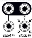
Clock and reset are analog logic *INPUT* and *OUTPUT* signals made to synchronize Ground Control together with other Eurorack gear (typical 1/16<sup>th</sup> notes clock and reset). The trigger outputs are 0...+10V range10 mSec length to be able to clock various gear. Trigger inputs are typically 0...+5V expected with the threshold of 0.65V.
