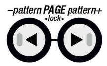
The main functions of these buttons is to switch the patterns on the active track, incrementing up or down with **◆** *PATTERN/PATTERN* **▶** buttons.
