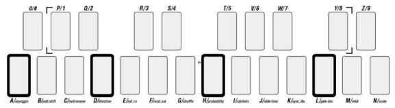
Sequencer has 2 octaves or 24 piano keys buttons – they are momentary, silicone rubber keys for entering melodies, drums, steps, selecting the patterns, accessing the menus, entering alphabetical and numerical values etc.
