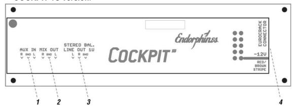
1. **AUX IN**: accepts audio input from other Mix Bus compatible modules and is basically another stereo input to be mixed with the rest 4 channels.
