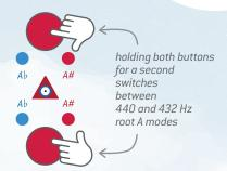
one blink at startup — 440 Hz root A:
